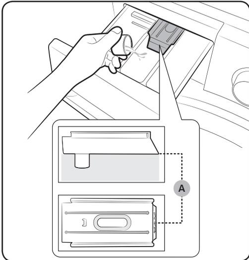
3. Aplique amaciante de roupa no
